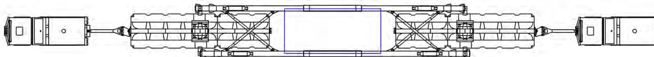
Plan view - 16 axle girder frame trailer - concept model only Indicative 160 te transformer Scale 1:200
